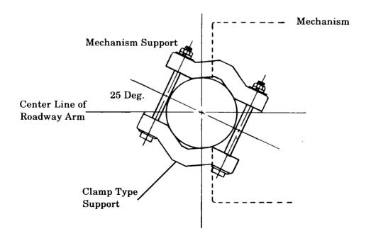
Clamp Type Mechanism Support Installation Part 3565-396
