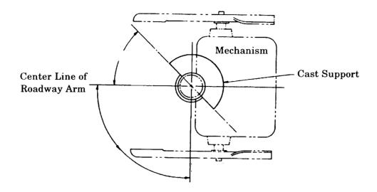
Cast Mechanism Support Installation Part 3565-380-A
